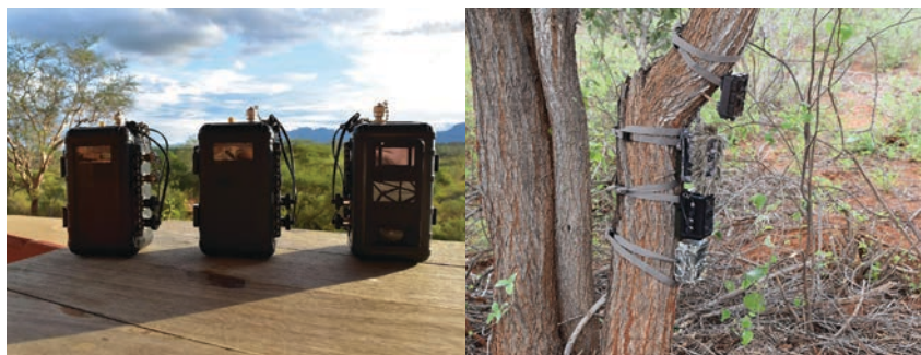
The system combines rugged cameras and sensors into a low-power radio network to monitor wildlife and detect human activity. The captured data is transmitted using satellite connectivity to Nominet's IoT Tools platform in the cloud, which is accessible to conservationists, helping them understand conditions on the ground, identify threats and develop methods to meet identified challenges
